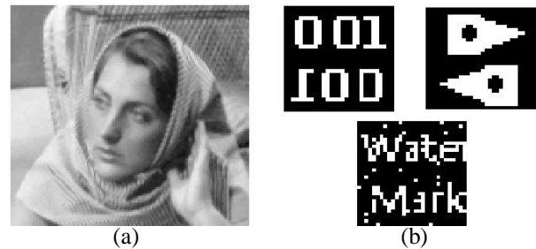
Fig.5. (a) The filtered watermarked image and (b) the extracted results
