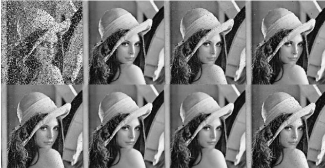
Fig 1: Results of different algorithms for Lena image. (a) Output of PSM. (b) Output of DBM. (c) Output of UTM. (d) Output of AM K=4. (e) Output of MDBUTM K=1. (f) Output of MDBUTM K=2. (g) Output of MDBUTM K=3. (h) Output of HDBF. Row 1 and Row 2 show processed results of various algorithms for image corrupted by 70% noise densities, respectively
