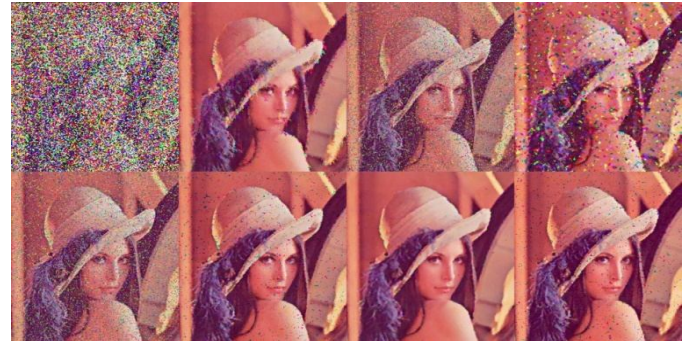
Fig 4: Results of different algorithms for Color Lena image. (a) Output of PSM. (b) Output of DBM. (c) Output of UTM. (d) Output of AM K=4. (e) Output of MDBUTM K=1. (f) Output of MDBUTM K=2. (g) Output of MDBUTM K=3. (h) Output of HDBF. Row 1 and Row 2 show processed results of various algorithms for image corrupted by 85% noise densities, respectively
