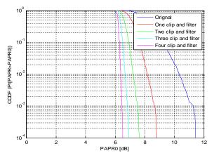
**Figure4**: PAPR reduction performance of original and Proposed ICF.
