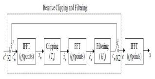
Figure 1: Iterative Clipping and Filtering scheme.
