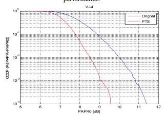
Figure3: PAPR reduction performance of original and PTS
