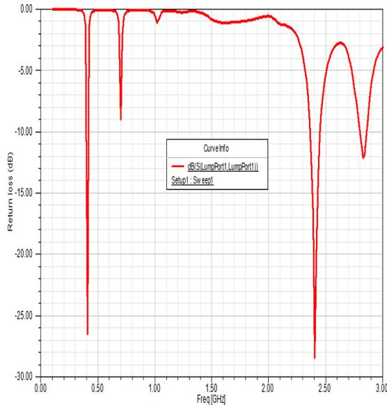
**Figure 2:** Simulated return loss for the MICS and ISM band
