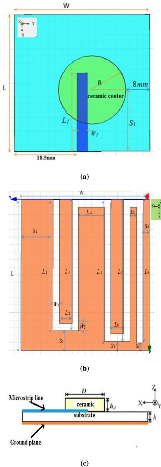
**Figure 1:** Proposed dual band DRA with serpentine slot: (a) Top view; (b) Bottom view; (c) Side view
