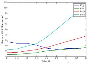
Figure 11: Variation in the Maximum RE Power of Section-1 and SE Power of Section-2 against k for diff. value of %S.
