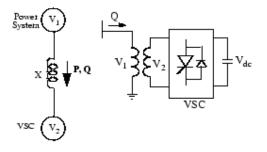
Figure 3: Schematic Diagram of Statcom
