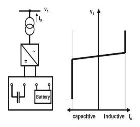
Figure 1: V-I Characteristics Of Statcom
