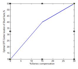
Figure 12: Optimal OFF-Center Location of Shunt Facts Device
