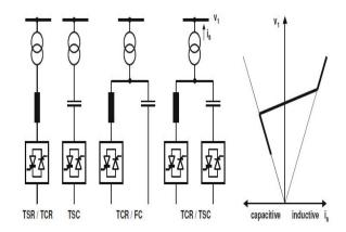
Figure 4: Schematic Diagram of SVC and V-I Characteristics.
