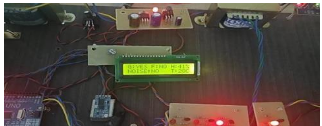
Figure 14: Gas Detected in Transmitter
