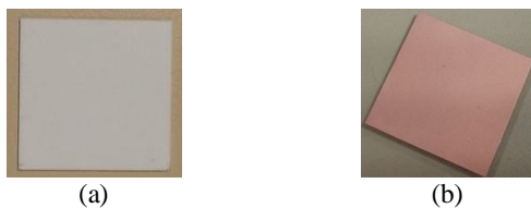
Figure 5: (a) Alumina substrate, (b) Alumina substrate by copper electroless plating.
