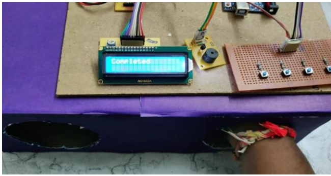
Figure 12: Completed message on the LCD display
