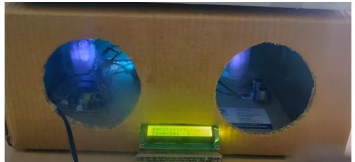
Figure 11: System setup with fog sanitizer, UV lamp and Ultrasonic sensor
