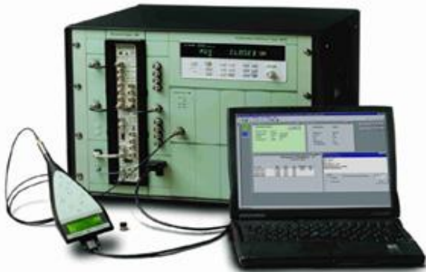
Figure 1: Platform B & K calibration system type 3630 A (Source: user manual of the system type 3630)
