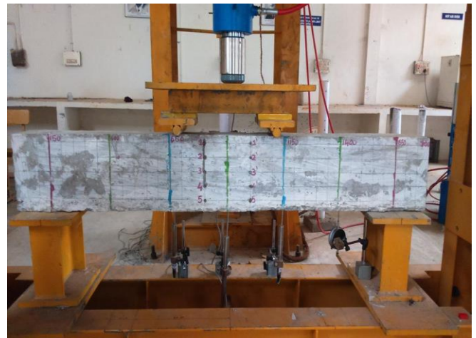
Figure 3: Loading frame setup
