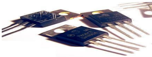
Figure: Voltage Regulators
