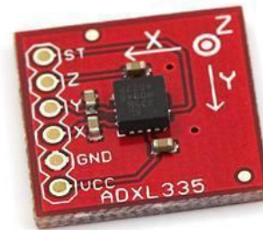
Figure.7 Triple Axis Accelerometer ADXL335
