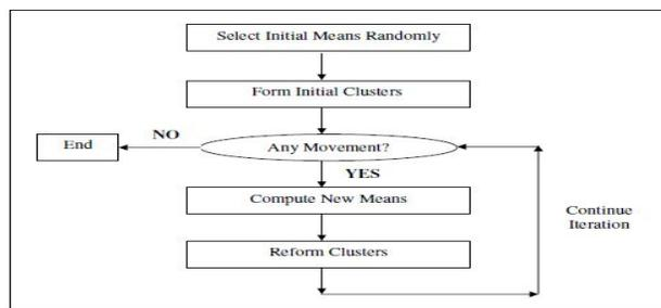
Steps of K-means Algorithm in Schematic Representation
