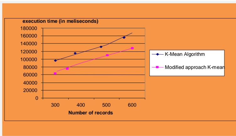
Graph shows the comparison between K-mean and Modified approach K-mean on the basis of large number of records and execution time using this algorithm. Modified approach K-mean better performance in comparison to standard K-means algorithm
