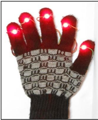
Figure 16. A glove used to assign red color to the fingertips using LEDs
