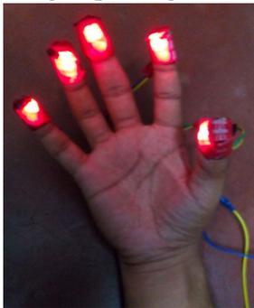
Figure 17. Finger-caps used to assign red color to the fingertips using LEDs
