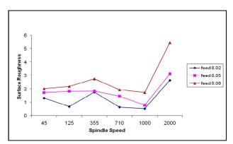
Fig 2 (b) – 6mm  $\phi$  Drill and different Feed Rates
