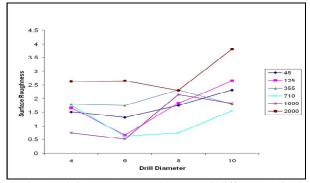
Fig 3 (a) – 0.02 mm/rev Feed Rate and different Spindle Speeds
