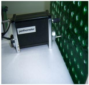
Fig: 1: Analysing surface roughness by Perthometer
