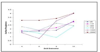
Fig 3 (b) – 0.05 mm/rev Feed Rate and different Spindle Speeds
