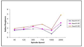
Fig. 2 (a) - 4mm  $\phi$  Drill and different Feed Rates
