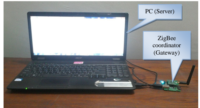
Figure 4: Implementation of the Master Station
