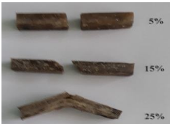
Figure 1: Specimen fracture due to Charpy impact test
