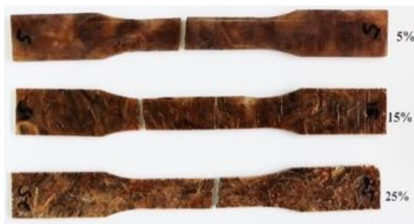
Figure 2: Specimen fracture by tensile test.
