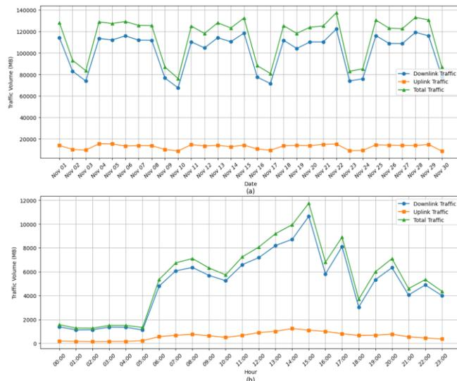
**Figure 2:** Traffic Volume Analysis for November 2025. **(a)** Monthly traffic trends from November 1 to November 30, showing uplink, downlink, and total traffic volumes. **(b)** Hourly traffic breakdown for November 15, displaying uplink, downlink, and total traffic volumes throughout the day.
