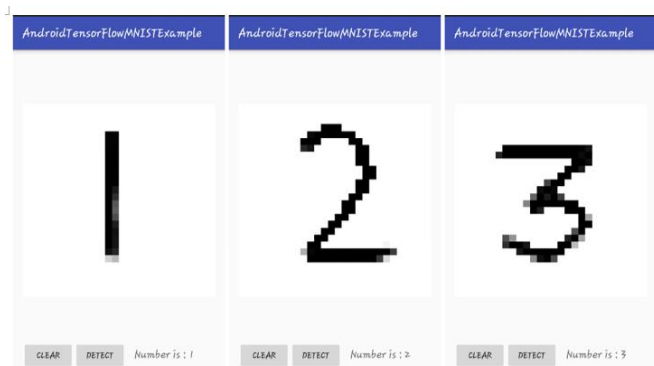
Figure 9: Deployed Model on Edge Device to Recognize Handwritten Digits
